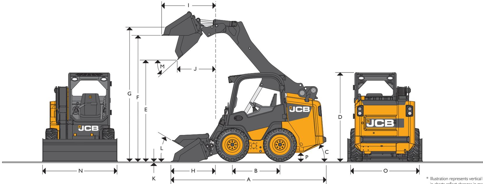
\* Illustration represents vertical lift machine. Specs in charts reflect changes in machines due to lift path.
