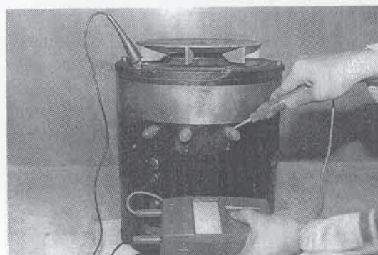
Measuring the Insulation Resistance
